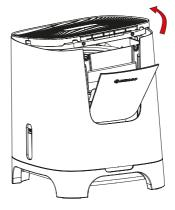
The grill will stay connected to the humidifier, rest it on the side.
